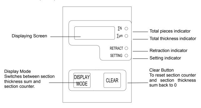
Fig. 5 main machine panel layout
